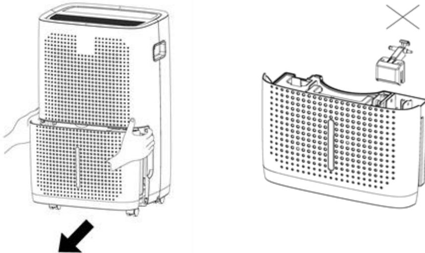
II. Empty the tank, then place it back in its proper position. Ensure that it is inserted correctly.
